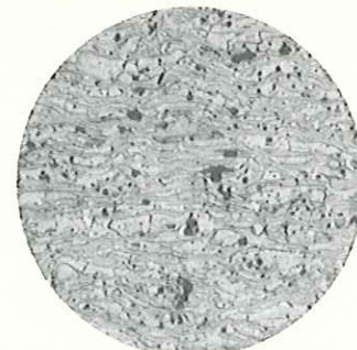
Spraying material : titanium oxide (100 magnifications)
